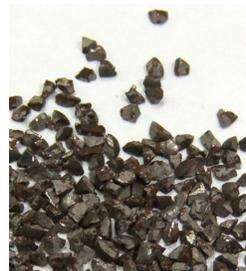
Steel Shot & Grit are durable metal abrasives that meet the requirements of Standard Specification 20-66 for Cast Steel Abrasives, published by the Steel Founders' Society of America.
