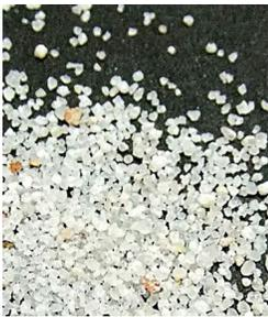
Lane Mountain Silica Sand is a high quality, high purity, close graded white silica sand. Lane Mountain Silica is also used as an additive for white plaster, mortar or concrete and industrial applications.
