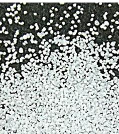
Soda blasting uses small sharp crystals of sodium bicarbonate (baking soda) that are propelled, by pressurized air or water, at a surface to remove coatings. Sodium bicarbonate is a food grade material that is non hazardous, water soluble, and won't damage most surfaces.
