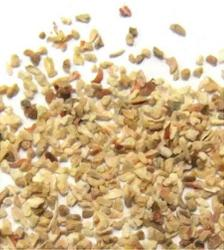
Corn Cob is the choice when the job calls for softer, less dusty and an environmentally safe abrasive. This blast cleaning media is suitable for metal, wood, fiberglass, plastic, masonry, electrical insulators and other sensitive materials. It is non-sparking and safe to use around gears and hydraulic rams. Corn Cob can be used in combustible environments (i.e. refineries).
