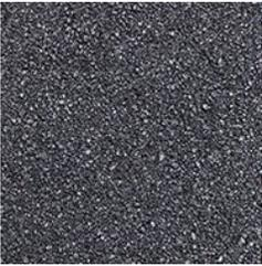
PRO-GRIT holds a solid place in the North American market because of its unparalleled quality. Recommended for cleaning rust, paint or scale on steel. PRO-GRIT features: Low dust emission, Cleans faster requiring less product. Contains less than 0.1% free silica.
