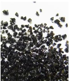
TARGET® Black Magic is an abrasive grit prepared by selective screening of coal slag to give a series of clean, sharp abrasives meeting the requirements of the abrasive blast cleaning industry.
