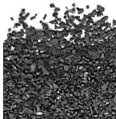
DURAMAX Abrasives® are a synthetic garnet made via world leading technology. With high compressive strength and Mohs hardness of 7.5, it is an ideal abrasive. The performance of garnet, at a fraction of the price. It is three times stronger than natural garnet so that your compressor's power is put to full use. Save your money with this high re-use abrasive (3+ times).
