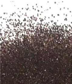
STARBLAST® blasting abrasives are a loose blend of coarse and fine staurolite sands that are uniformly sized and have clean, rounded surfaces. Mined from mineral deposits in Northeast, Florida, the naturally occurring sands are scrubbed and chemically washed to ensure freedom from dirt, dust, and ultrafines. This product is approved by the California Air Resources Board for use in dry, unconfined blasting operations.
