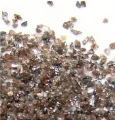
Aluminum Oxide grits are the most efficient blasting media. It is the fastest cutting product used for industrial blasting and surface preparation, due to its extreme hardness of 9 on Moh's scale. Aluminum Oxide is a manufactured material, electrofused from bauxite. Grit sizes available: #16, #24, #36, #54, #70, #100, #220
