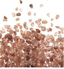
Garnet is a naturally occurring almandite garnet, the hardest of all known garnet types. All grades have a Moh's hardness of 8, with a specific gravity of 4.1. Garnet is available in size grades to meet requirements for any project. Grade sizes are: 12-25, 20-40, 30-60, 50-80, #80.
