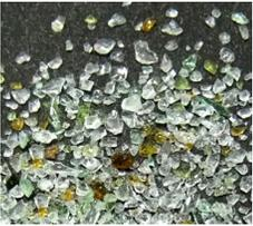
Glass Abrasives are clean, high quality, close graded, processed, crushed, recycled glass. Grade sizes available are: 10-30, 12-50, 30-60, 50-100.
