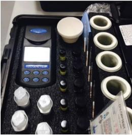
**CHLOR\*TEST "CSN Salts"** offers the specifier the availability of trouble-free performance testings, in the field, for chlorides, sulfates, and nitrates from *one* extraction.
