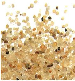
TARGET® Silica Abrasives are high quality, close graded silica sands which undergo up to three washings to provide a clean, high quality material. Target Silica Abrasives are suitable for sandblasting of steel, concrete or wood in preparation for coating or repair, to obtain architectural effects in concrete or wood, an aggregate for cementitious or polymer grouts, mortars and concrete and for foundry mold sand, traction sand and industrial sands.
