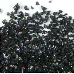
Kleen Blast is prepared by selective screening of copper slag to give a series of clean, sharp abrasives meeting the needs of the abrasive blast cleaning industry. The product is approved by the California Air Resources Board for use in dry, unconfined blasting operations.
