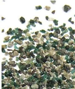
TARGET® Green Diamond Abrasive Grits are high efficiency blasting grits prepared by selective screening of nickel slag. These gradations are available to provide materials suitable for most blast cleaning operations. All grades have a Mohs hardness of 7, giving improved cutting and productivity relative to conventional industrial and silica sands. The product is approved by the California Air Resources Board for use in dry, unconfined blasting operations.
